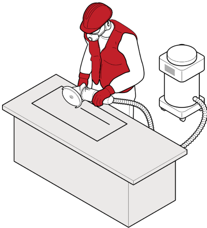
Figure 5 A worker cutting/grinding with on tool dust extraction
