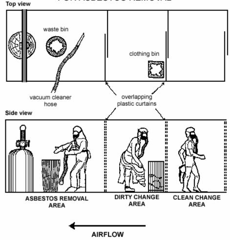
Figure 4 - Typical Layout of a Mini-Enclosure
