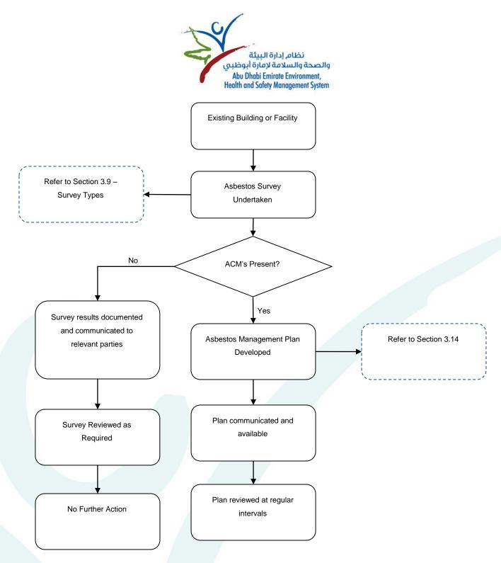
Figure 1 - Identification of Asbestos -All Non Domestic Buildings / Facilities
