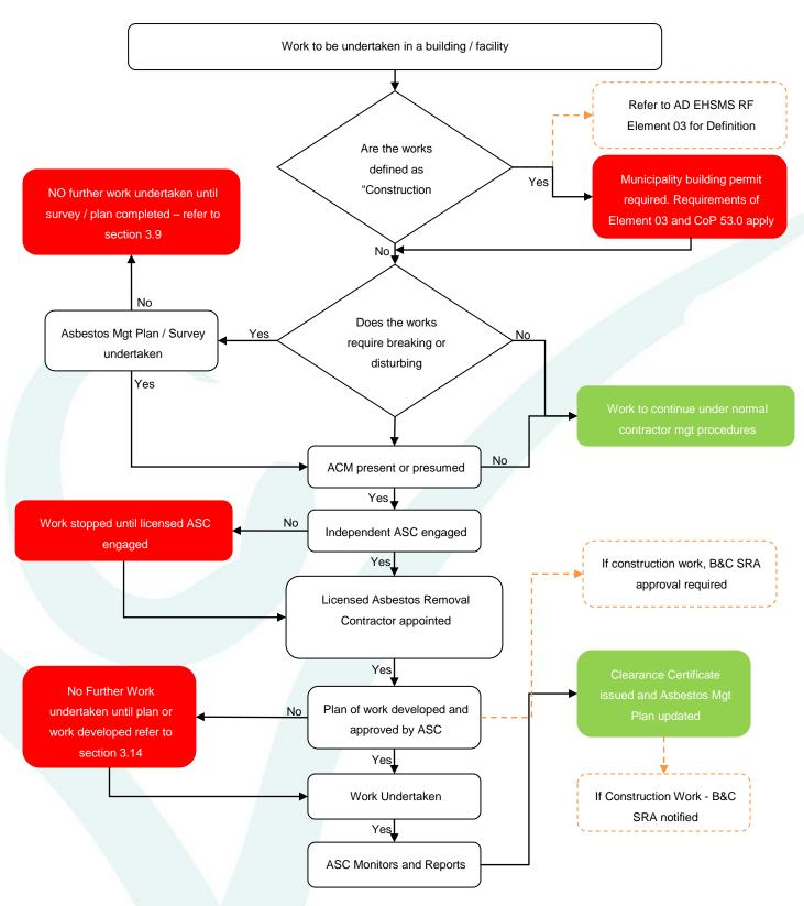
Figure 2 - Working with Asbestos
