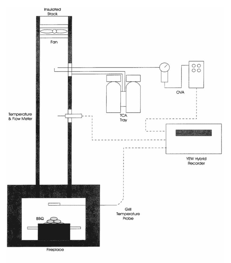
Figure 3. Sampling Apparatus Set-up with Chart Recorder
