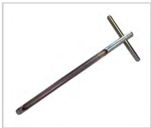
Figure A6-3: Soil Auger/Corer
