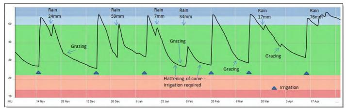
Figure 5-1 Weighted average soil moisture content (to a depth of 80cm) measured with a capacitance probe under surface irrigated lucerne (Soil Moisture Monitoring factsheet, Agriculture Victoria, December 2017)
