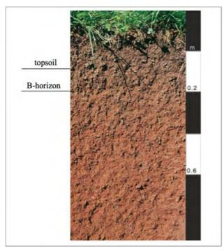
Figure A6-1: CROSS SECTION VIEW: sample soil profile showing horizons and areas for sampling
