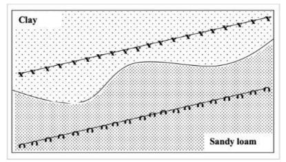
Figure A6-2: PLAN VIEW: sample paddock with two different soil types and transects showing locations of topsoil sub-samples
