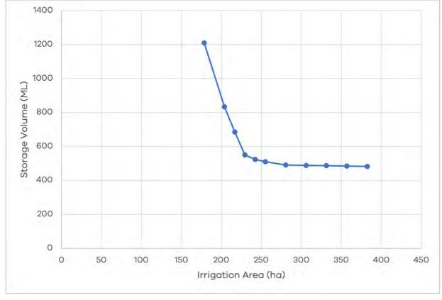
Figure A1-1: Water Balance Model – Example Output of Irrigation and Storage Combinations
