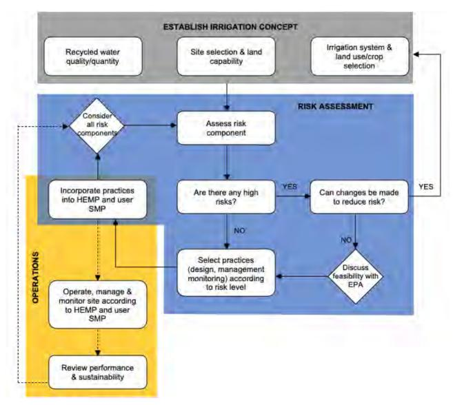
Figure 2-4 Assessment Process for Recycled Water Irrigation Schemes
