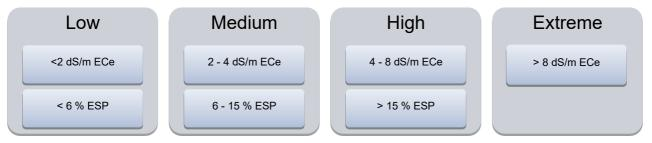
Figure 6-2 Soil salinity and sodicity risk assessment (ESP = exchangeable sodium percentage, ECe = Electrical conductivity of the soil extract)
