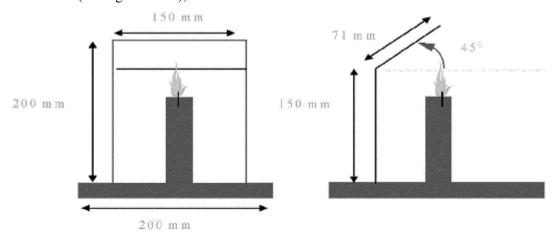
(e) the candle placed on the metal support shall be positioned midway between the two ends of the drum (see Figure below);
