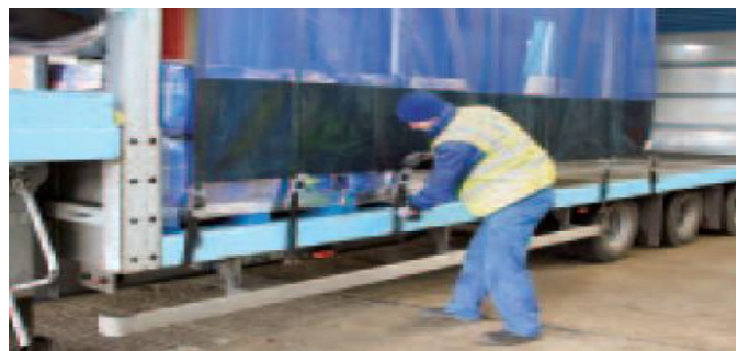
Figure 6-14: Secure Dangerous Goods to the Vehicle
