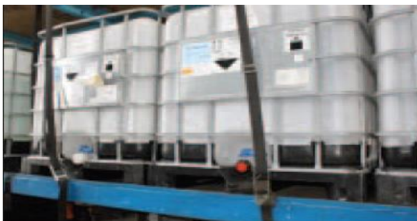
Figure 6-14: Secure Dangerous Goods to the Vehicle
