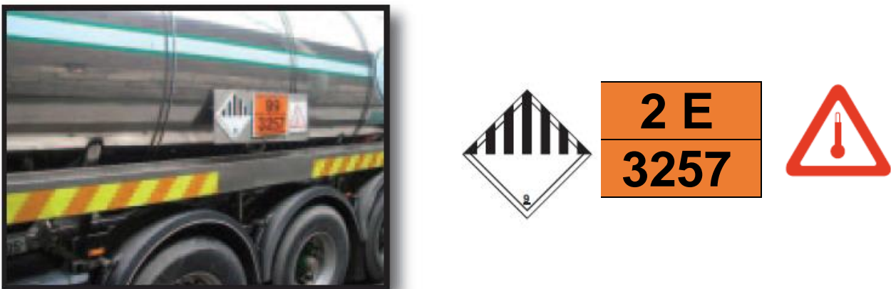
Figure 6-7: Tank Marking and Labelling
