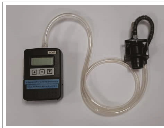
Figure 9: Sampling Train for Respirable Fibres
